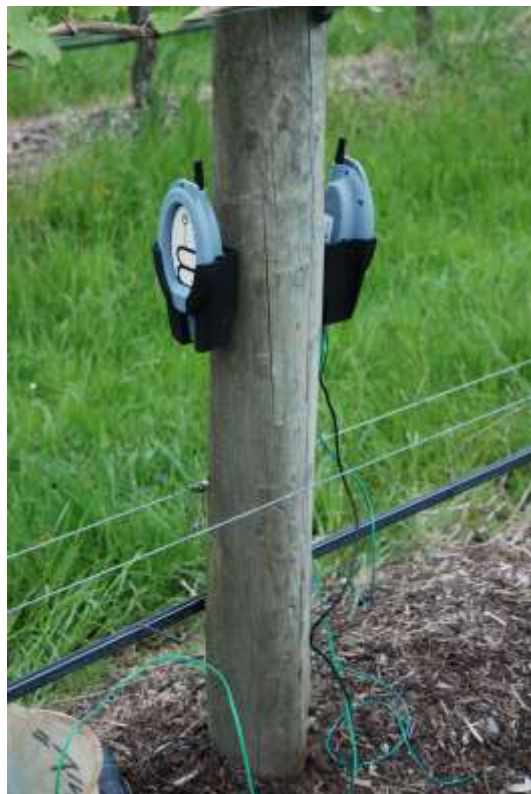
Figure 3: The Carta sense soil moisture and temperature monitoring device
